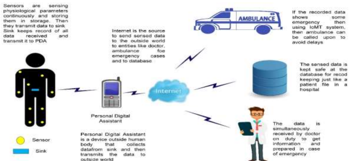
Figure 3. Architecture of loHT
